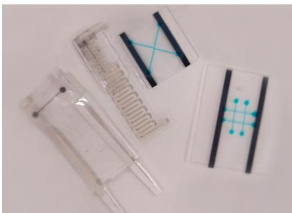
Different types of microfluidic pressure sensors
